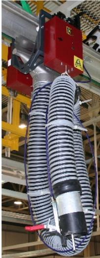
Automatic Hose Trolley with Drive Unit and Motorized Hose Lift
