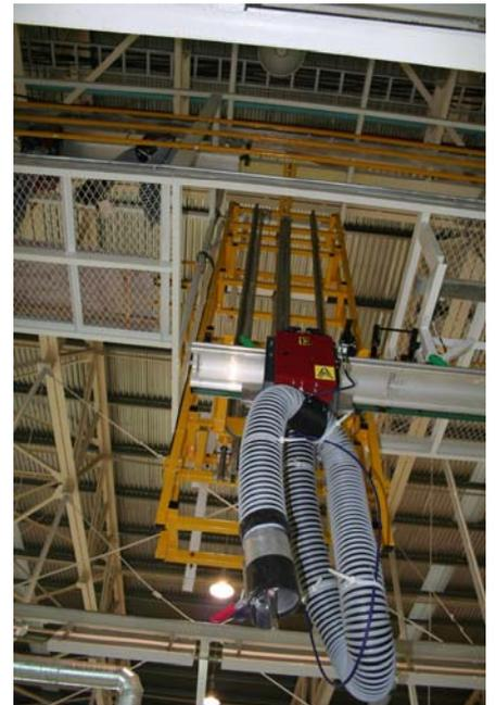
Full Automatic Vertical Shifter ensure the transfer of the hose trolleys between two return rails located at different levels. Facilitates an ergonomic installation into the automotive factories. Maximum safety due to two-ways locks, limit switches and overload protection.
