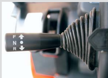
Simple, Small-Stroke F/R Lever The forward-reverse lever swings through a smaller arc than previous models, meaning less effort and less total time used during this basic, often-performed function.
