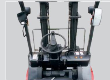
Wide-View Mast The operator is able to work with increased safety and accuracy due to a wider view mast.
