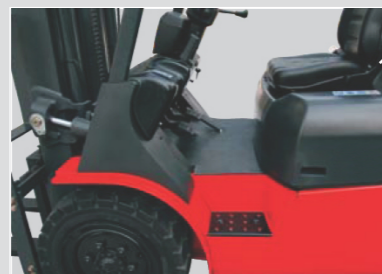
Wide-Open Operation Space The area between the foot pedals and the body below the seat is open and free of obstructions that hamper entering and exiting the forklift.
